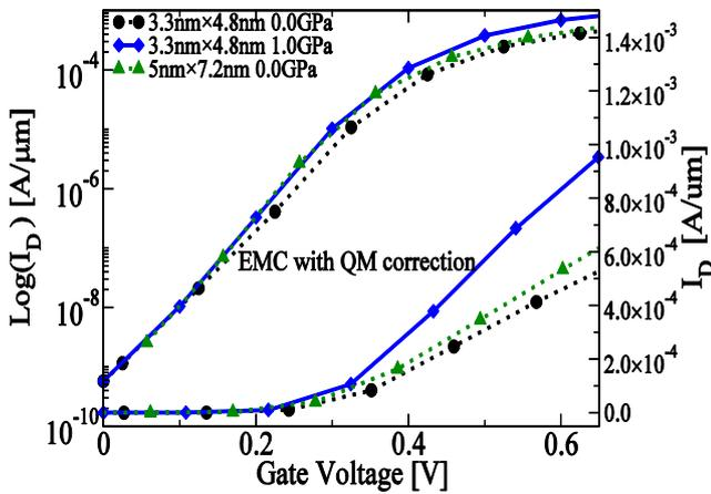
Fig3  $I_D$ - $V_G$  characteristics for 3.3nm x 4.8nm cross-section with and without strain compared with unstrained 5nm x 7.2nm normalized by (equivalent pitch) and aligned at leakage current ( $I_{off}$ )  $6 \times 10^{-10}$  A/um by employed Poisson-Schrödinger with MC.
