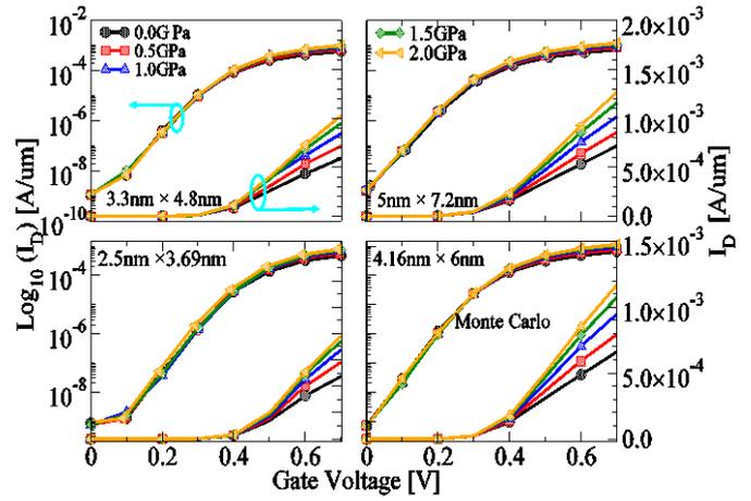
Fig.4  $I_D$ - $V_G$  curves for four different applied strain on elliptical Si NWT with four different cross-section dimensions: 5nm x 7.2nm, 4.16nm x 6nm, 3.3nm x 4.8nm, and 2.5nm x 3.69nm. All results are normalized by pitch length.
