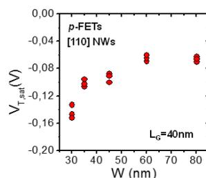
$V_{T,sat}$  vs  $W$  for stacked-NWs *p*-FETs with  $L_G=40\text{nm}$  at  $V_{DD}=0.9\text{V}$ .
