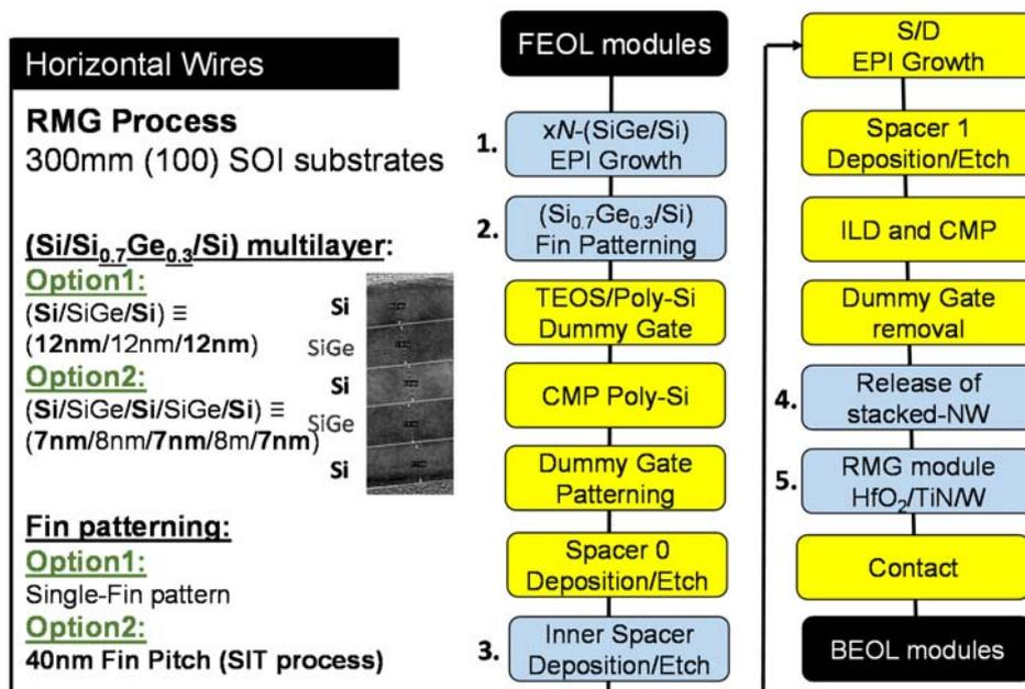
Inner spacers and SiGe:B raised-S/D are used. The Ge concentration in the SiGe layers is around 30%. The steps numbered '1' to '5' are specific technical requirements for stacked wires FETs (as compared to FinFET devices)
