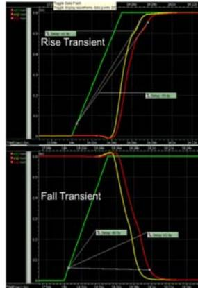
NAND-based latch circuit with and w/o RC
