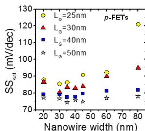
Subthreshold slope vs wire width ( $W$ ) for stacked-NWs *p*-FETs with  $25\text{nm} \leq L_G \leq 50\text{nm}$ .
