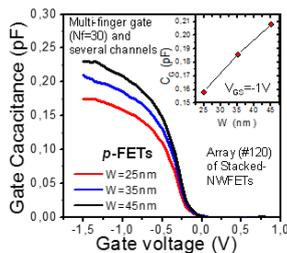
Gate capacitance vs  $V_{GS}$  for stacked-NWs *p*-FETs with  $W=25-45\text{nm}$ . Here,  $L_G=500\text{nm}$ .
