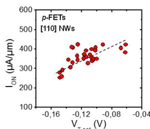
$I_{ON}$  vs  $V_{T,sat}$  for stacked-NWs *p*-FETs with  $W=25-35\text{nm}$  at  $V_{DD}=0.9\text{V}$ .  $25\text{nm} < L_G < 70\text{nm}$ .
