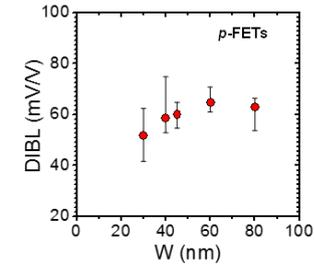
Median DIBL vs nanowire width ( $W$ ) for stacked-NWs *p*-FETs with  $L_G=40\text{nm}$ .
