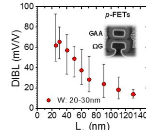
Median DIBL vs gate length ( $L_G$ ) for stacked-NWs *p*-FETs with  $W=20\text{nm}-30\text{nm}$ .
