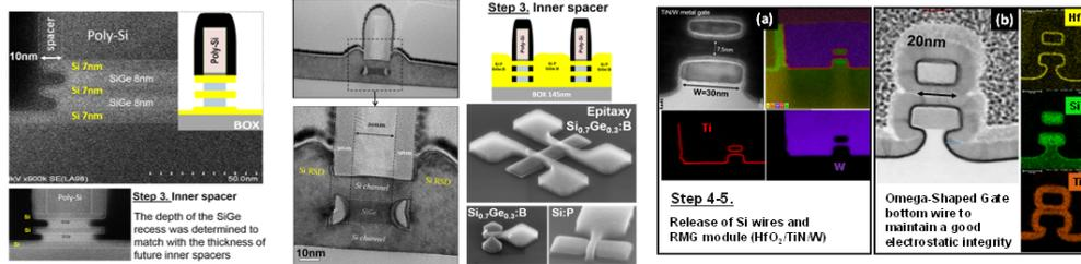
Cross-sectional SEM images of stacked-NWs FETs prior to SiN inner spacers integration. The Si and SiGe thicknesses are 7 nm and 8 nm, respectively. The etching of SiGe layers stops at the same 'x' position than the spacer/poly-Si dummy gate interface.
