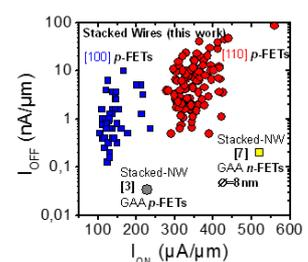
$I_{ON}/I_{OFF}$  plot of [100] and [110] stacked-NWs *p*-FETs with  $W=20\text{nm}-30\text{nm}$  at  $V_{DD}=0.9\text{V}$ .
