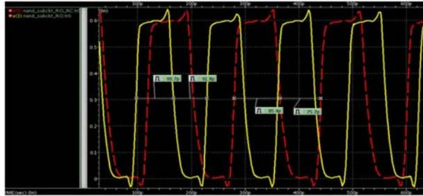
NAND-based ring oscillator with and w/o RC
