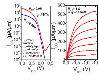
$I_{DS}-V_{GS}$  and  $I_{DS}-V_{DS}$  characteristics of stacked-NWs *p*-FETs with  $L_G=25\text{nm}$ . Here,  $W=30\text{nm}$ .
